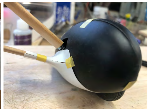
Spats assembled showing undercarriage transition.
