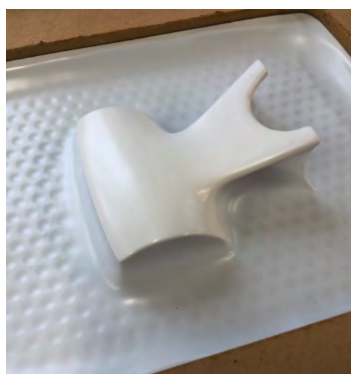
Vacuum formed under section from leg to spat.
