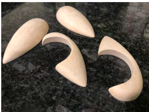
ABOVE: Plugs for spat vacuum forming.
