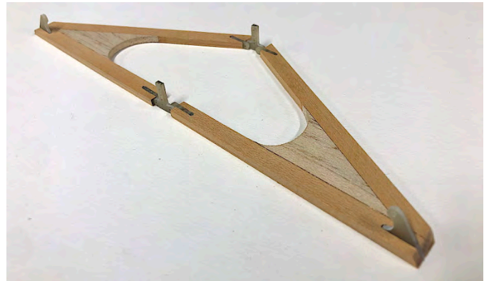
ABOVE: Undercarriage showing leg connection points and also the Compression strut.
