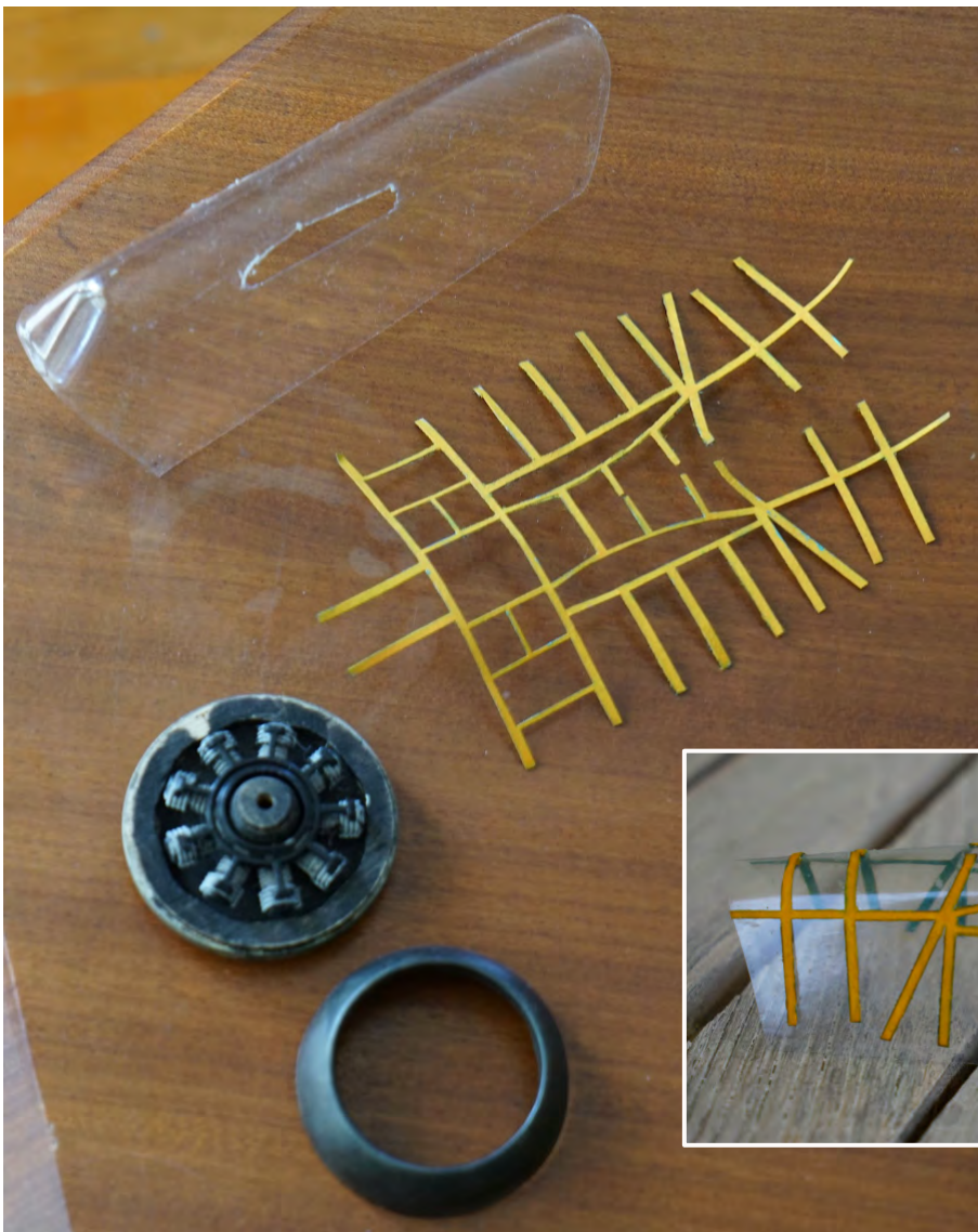
TOP: The framework prior to covering, showing the laminated undercarriage legs and wheel spats.
