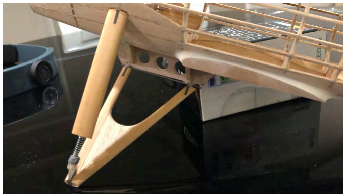
ABOVE: Undercarriage showing leg connection points and also the Compression strut.
