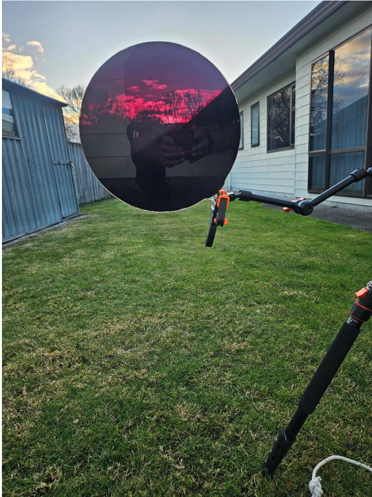
Tripod sun paddle Made up with Perspex or plexiglass and window tint
