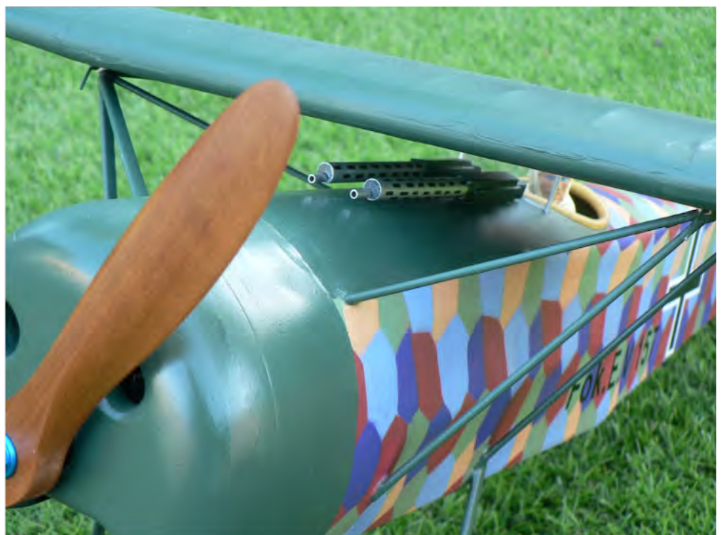
ABOVE AND RIGHT: Views of the DVIII showing the lozenge markings. Under wing hooks show that the wings are fixed with internal rubber bands. Machine guns are visible under the centre-section.
