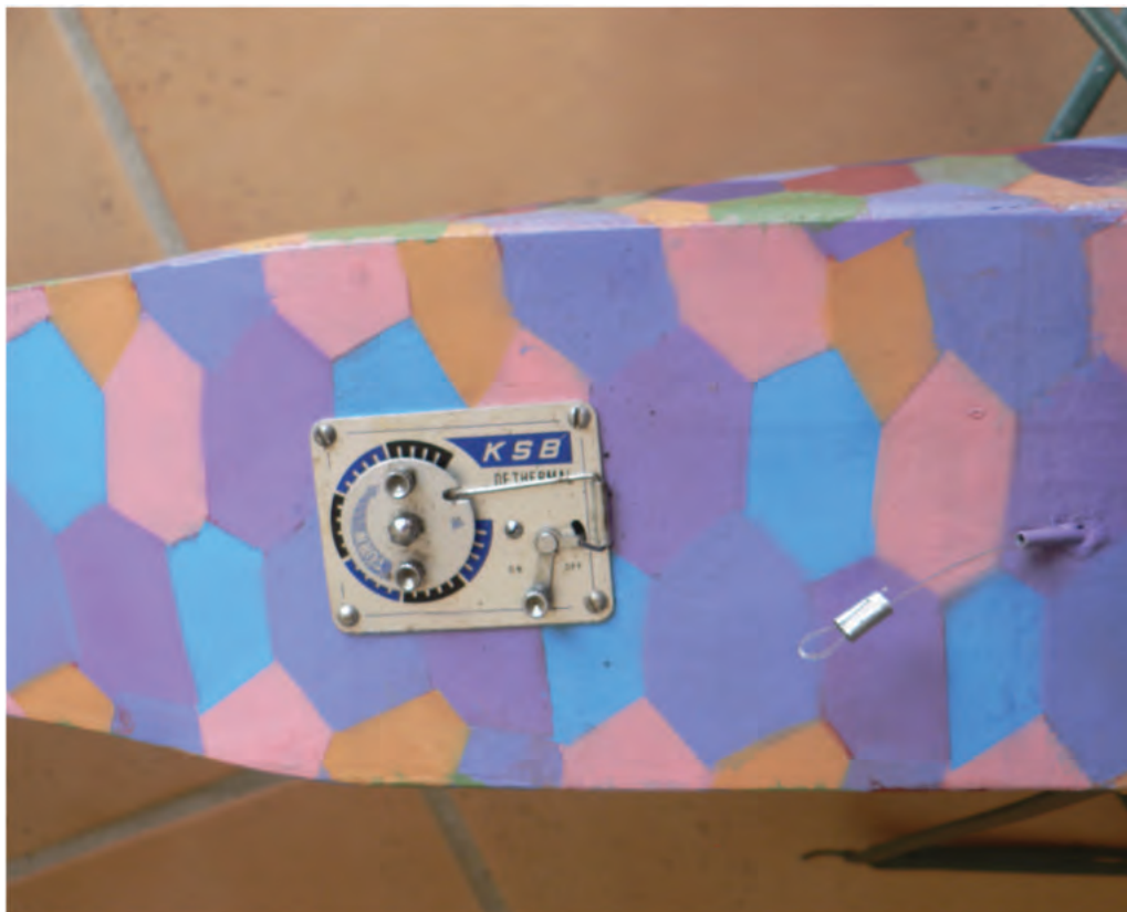
LEFT: A view of the KSB engine timer set-up and the lozenge scheme under the fuselage.
